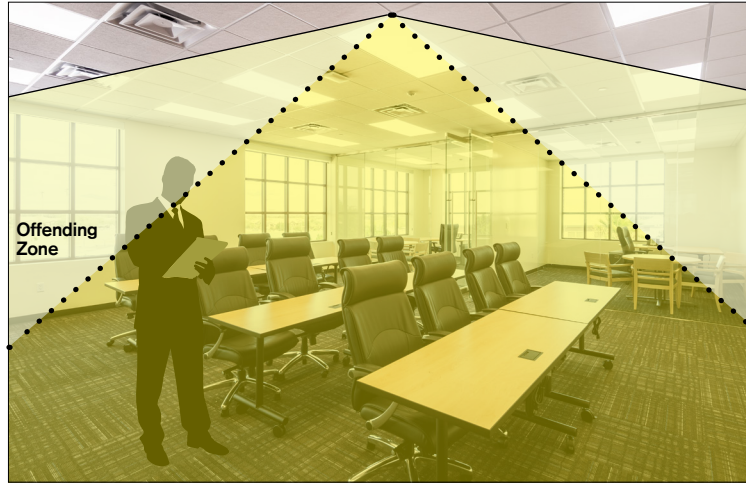
□ = Volumetric flat panel with micro-prismatic lens will reduce glare going into the occupant's eyes — = 90° ..... = 60°
